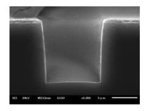
Rate = 560nm/min Pattern Width =  $10 \mu$ m Depth =  $11.2 \mu$ m
