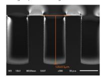
Rate =  $18 \mu$  m/min Pattern Width =  $50 \mu$  m Depth =  $128 \mu$  m
