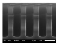
Pattern Width =  $4 \mu$  m Depth =  $10 \mu$  m Rate =  $1.25 \mu$  m/min
