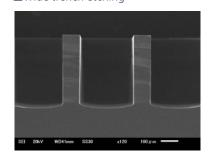
Pattern Width =  $300 \mu$  m Depth =  $420 \mu$  m Rate =  $6.4 \mu$  m/min
